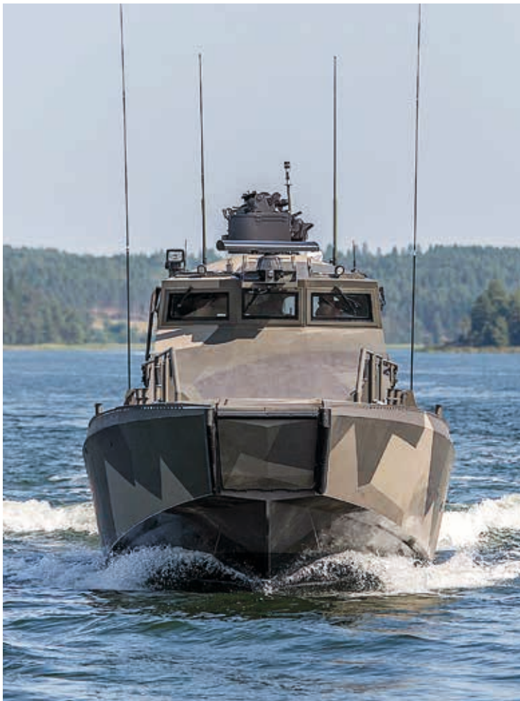
BELOW: The Watercat M18 AMC is propelled by two Rolls-Royce Steel series 40A3 waterjets, which give it a fully-loaded top speed of over 40 knots.
