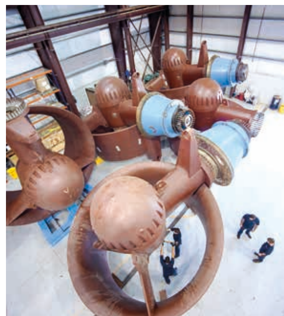
RIGHT AND ABOVE: The Galveston workshop is capable of overhauling multiple large azimuth thruster units.
