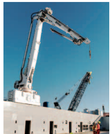
Dual draglink cranes allow fast and safer loading, unloading and moving of cargo over the entire length of the main deck.
