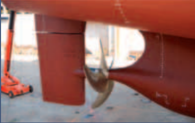
A typical Promas newbuild installation, showing the twisted rudder.
