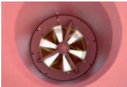
Permanent magnet tunnel thrusters are resiliently mounted in the tunnel to minimise noise and vibration. Installation and removal can be carried out without drydocking the vessel.
