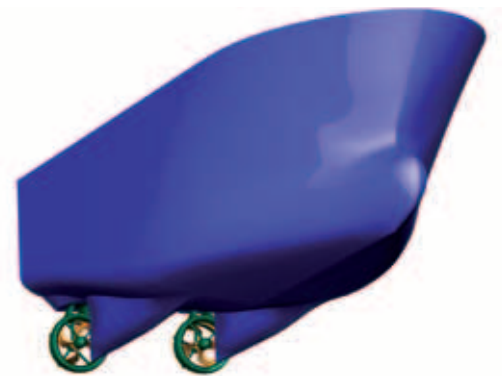
Technology demonstrator PM steerable nozzles or azimuth thrusters with a rating of 500kW are being installed on the research vessel Gunnerus .
