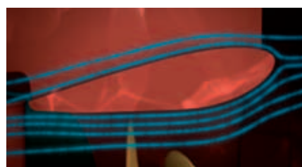
The Promas nozzle in a free-running situation, showing the profile controlling the water flow to minimise drag.
