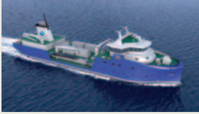
The NVC 386 can transport up to 450 tonnes of live fish in cargo holds equipped with sliding bulkheads and a pressure system for loading and unloading.
