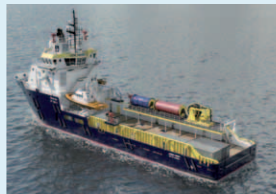
The UT 535 E can remain on site for extended periods, carrying out oil skimming operations.
