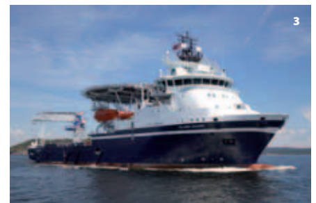
3. The longest variant of the successful UT 776 CD family of designs, Island Crown has a large accommodation unit and is fully equipped for other offshore roles.
