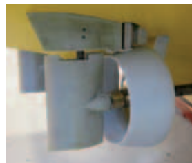
CFD calculations have been confirmed by tank testing with large-scale models (centre) and at the Rolls-Royce Hydrodynamic Research Centre (right).
