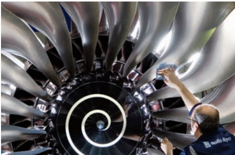
Technology creating global opportunities: Trent 1000 The front fan of a Trent 1000 engine showing its swept wide-chord blade design. The Trent 1000 is the launch engine for the new Boeing 787 Dreamliner aircraft.
