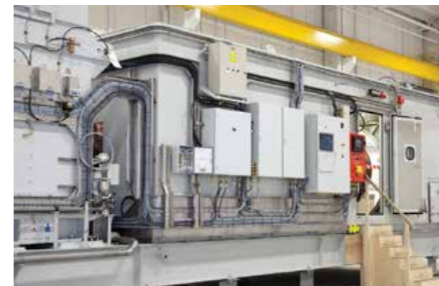
The MT30 alternator packages which powers the Royal Navy's Queen Elizabeth class aircraft carriers and the US Navy's DDG 1000 destroyers.
