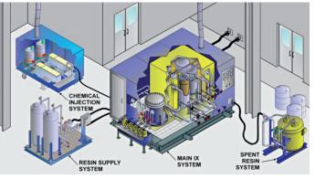
Using an AECL patented decontamination process, Rolls-Royce designed and supplied this custom system to reduce radiation emissions from the process piping in the NRU reactor at AECL's Chalk River Laboratories facility.
