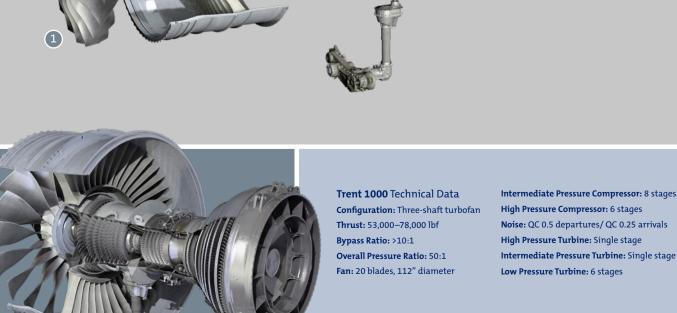
Noise: QC 0.5 departures/ QC 0.25 arrivals High Pressure Turbine: Single stage Intermediate Pressure Turbine: Single stage Low Pressure Turbine: 6 stages
