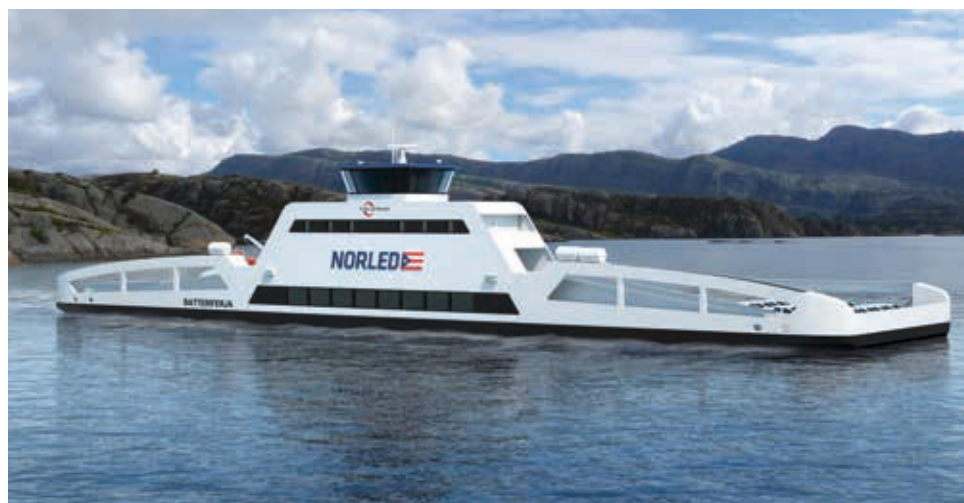
BELOW: The ZeroCat 120 battery-powered ferry will have space for 120 cars and up to 360 passengers.
