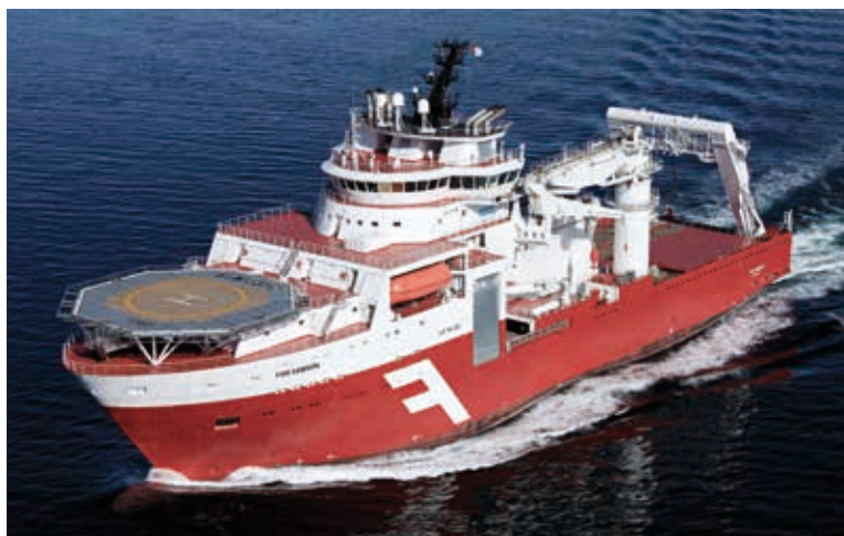
TOP: The UT 712 anchorhandling vessel Olympic Octopus was the world's most innovative when it entered service in 2006, with an array of safer deck equipment, DP2 and automation.
