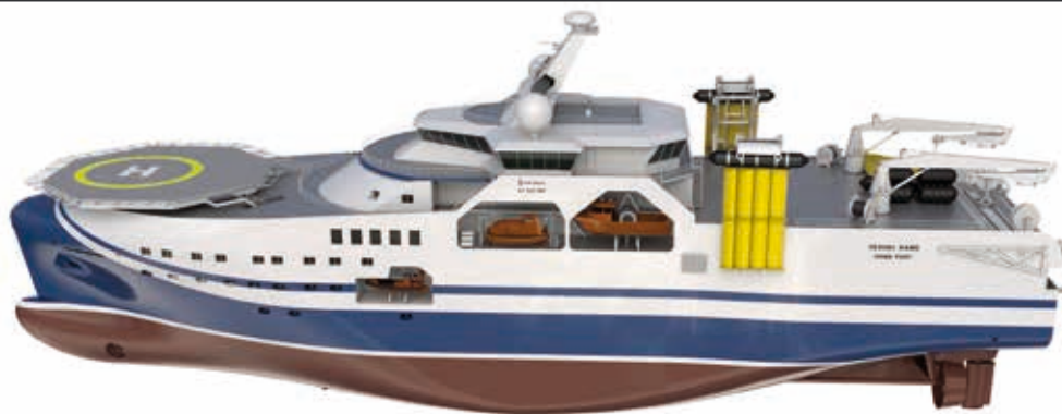
ABOVE: The efficient UT 833 with up to 180 tonnes of towing force gives a highly competitive fuel cost per square kilometre surveyed.
