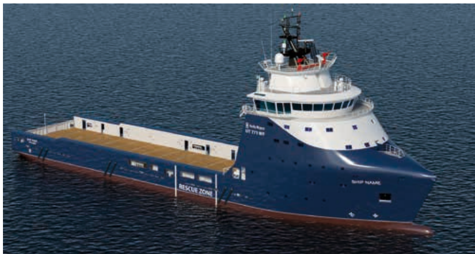
BELOW: The UT 771 WP complements other PSV designs and can carry a range of cargoes in a safe and efficient way. It has a deadweight of 4,200dwt.
