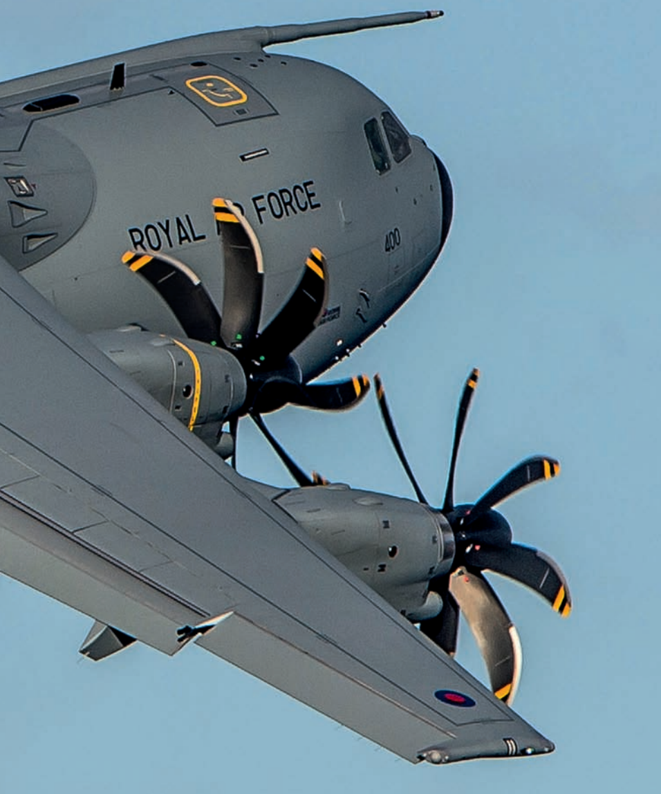
The A400M is powered by four TP400 turboprops. The scale of the engine can be seen (left).
