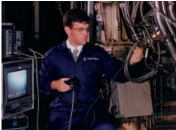
Borescope inspection provides in-service health assessment
