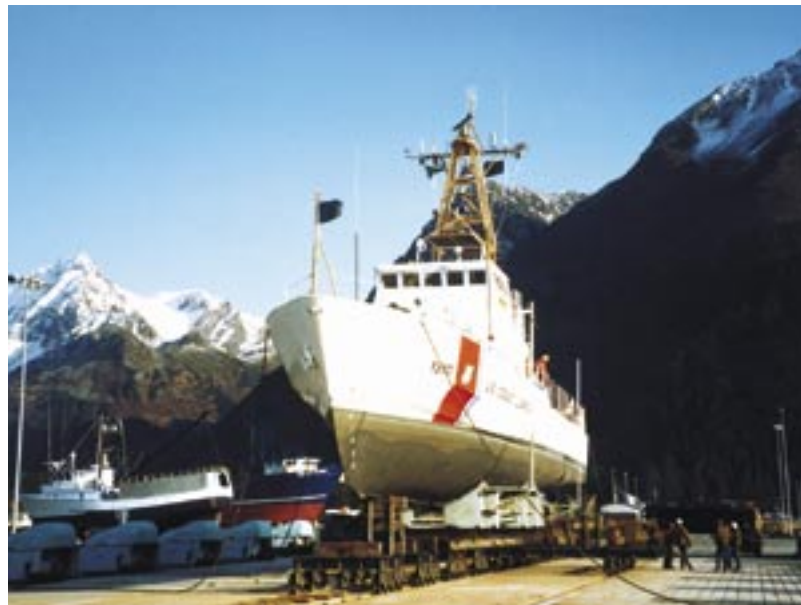
US Coast Guard vessel on a Syncrolift® Shiplift and Transfer System at Seward, Alaska
