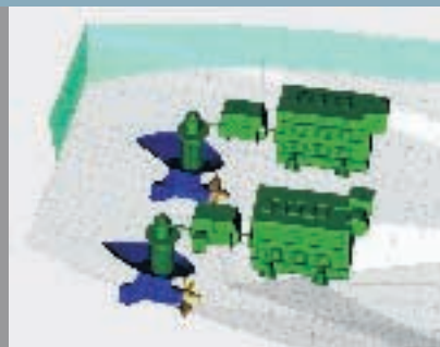
Two independent propulsion lines ensure redundancy
