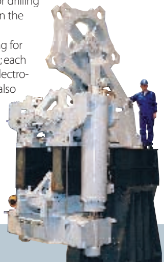
One of 16 chain jacks for 171mm chain with turn down sheave
