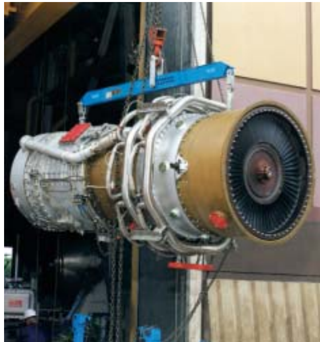
Avon DLE gas generator
